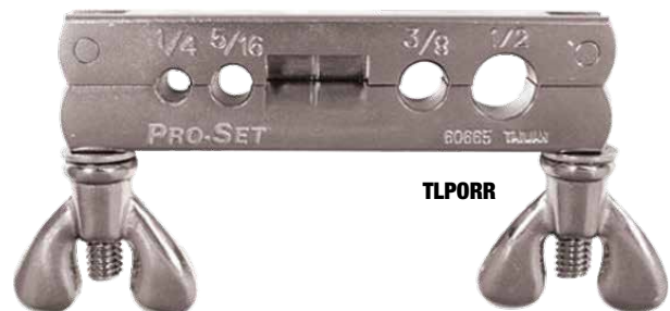
PRO-SET® PINCH-OFF & RE-ROUND TOOL Pinch-Off tool & rerounds 1/4", 5/16", 3/8", and 1/2" copper and tubing
